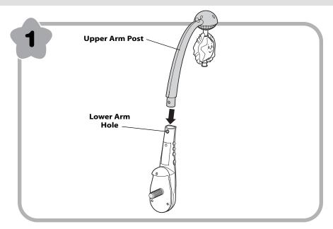
• Fit the post on the upper arm into the hole in the lower arm as shown.
